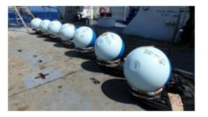
Last May, researchers embarked on the oceanographic vessel « Pourquoi Pas? » released at sea twenty drifting buoys which allow to study the sea surface temperature and the ocean currents at 15m depth. The journey of these buoys is followed in real time by a GPS satellite positioning system.
