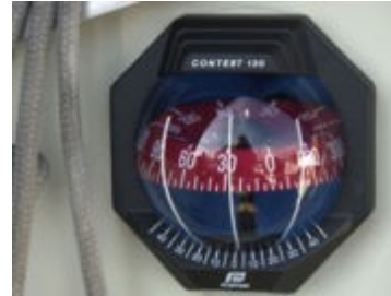
Sailboat compass with sphere (reading from side).
