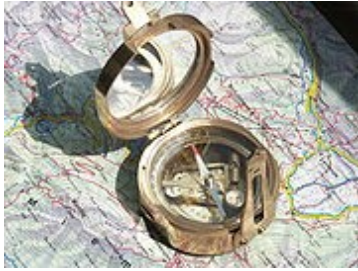
Marine compass with built-in inclinometer and spirit levels
