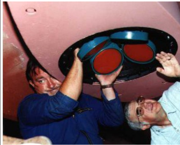
Attaching the hull-mounted ADCP
