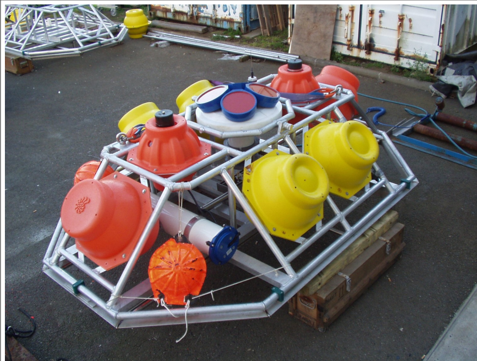
Example of a bottom-mounted mooring (Ifremer, Ecolophy 2005) with floats that allow it to ascent to the surface.
