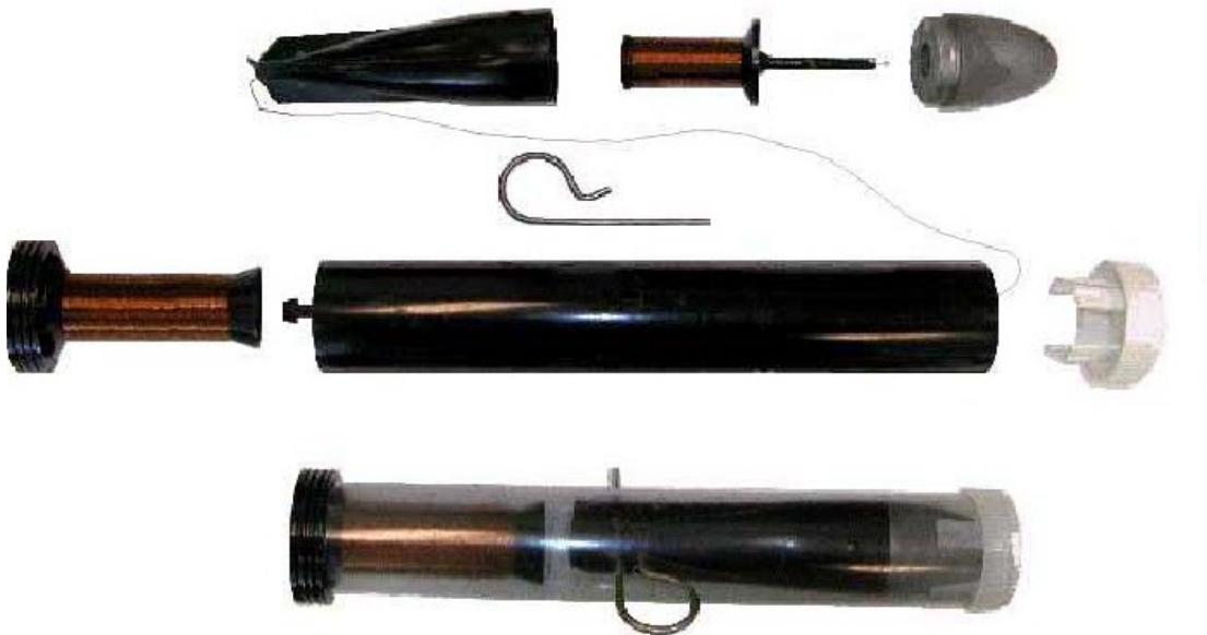
Figure: Various XBTs. Top: exploded view of a socket and probe; bottom: fully assembled.
