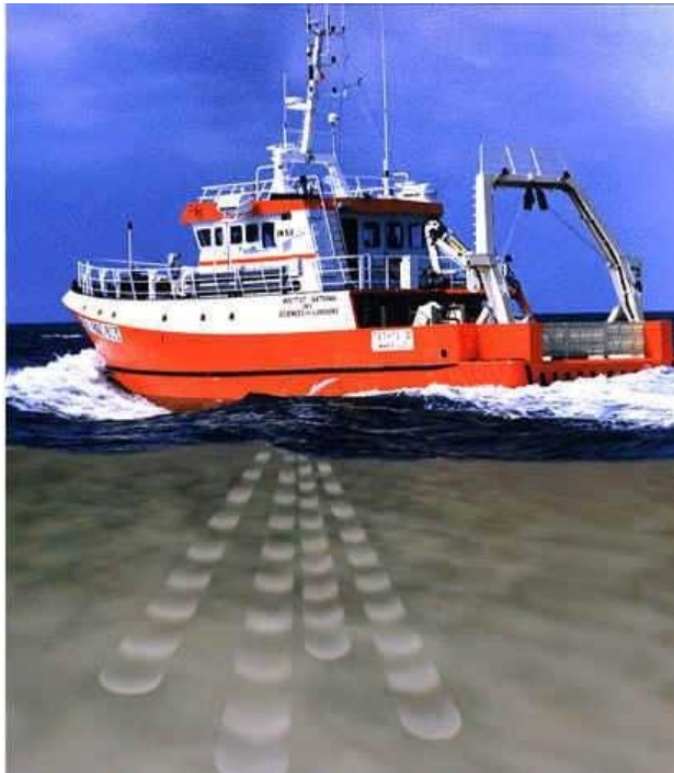
Acoustic measurements using the ADCP
