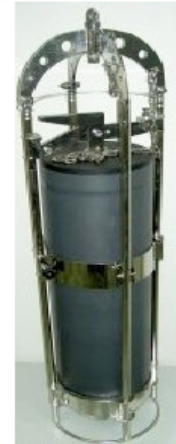
NPA (Systea) (nutrient probe analyzer)
